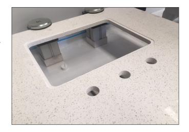
Pieces are held in place during processing by a series of pneumatic clamps and supports.
