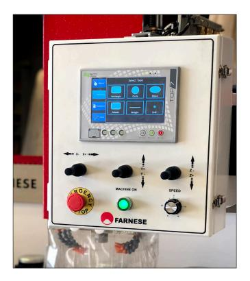
The **EASYSINK** boasts a predefined sink library of over 200 sink types ( taken from the bigger Alexia model), making it easier and more efficient to program a sink cutout.
