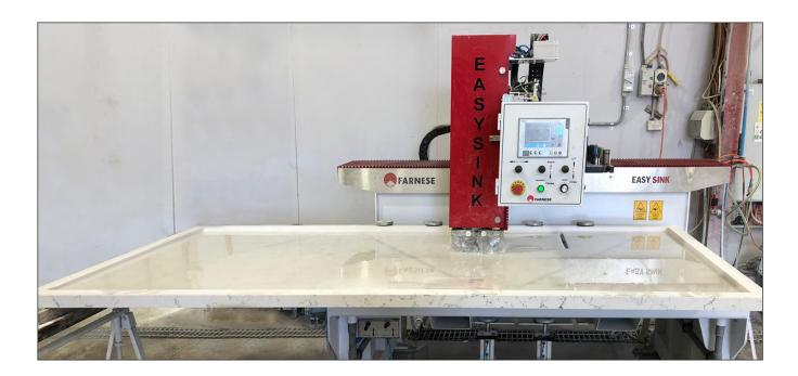
The **EASYSINK** allows for increased productivity in your factory, taking around 8 -10 minutes to cut out a 300mm x 400mm sink, or around 28 - 30 minutes to cut and polish.
