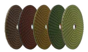
These are the resin pads we supply in our Top Polish Kit. They produce a superior quality polish with excellent clarity on most true granite and quartzite. They polish at low speed (in a home) or high speed (in a shop) with very minimal down pressure but must be kept wet at all times. These pads eliminate the old wet-to-dry top polishing method and simplify the top polishing process, yielding amazing results. Available in 5 grits - 200, 500, 1000, 2000, & 3000.
