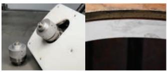
Finish grind with coarse drum wheel followed by the fine drum wheel to produce an easy to polish edge
