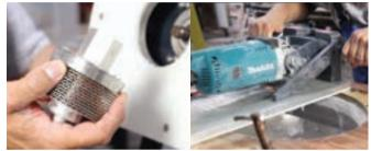
Attach Rapid Z<sup>™</sup>-CUT and grind sink to the template
