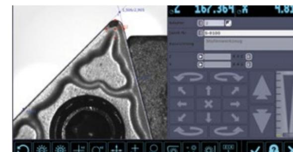
Cutting tool inspection in »pilot 1.0« software
