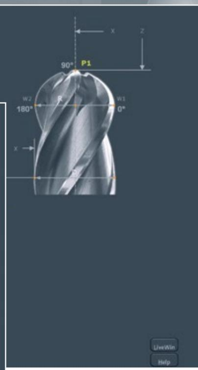
Measuring program 137: For fully automatic determination of the radius contour.
