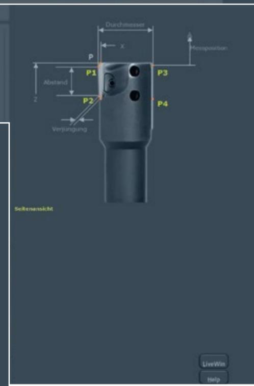
Measuring program 1: For the measurement of single-blade reamers with support strip in snap gauge principle.
