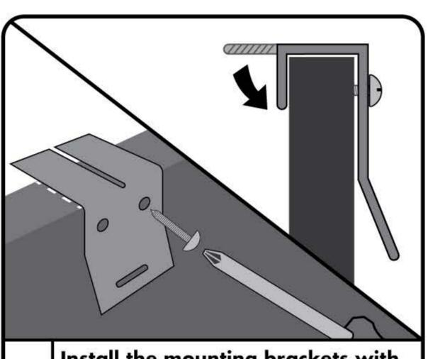
Install the mounting brackets with the provided screws. Bend the mounting tabs down over the cabinet divider for added strength.
