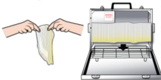
Remove membrane from outer plastic shipping bag. Unfold membrane & place into the rack. Wash hands after handling membranes.
