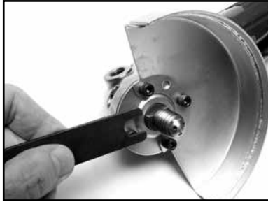
(J) Place wrench on bottom of spindle.
