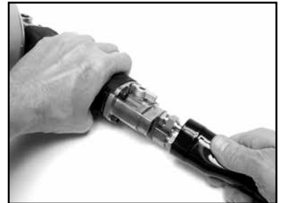
(F) Slide the exhaust hose over the water and air hoses.
