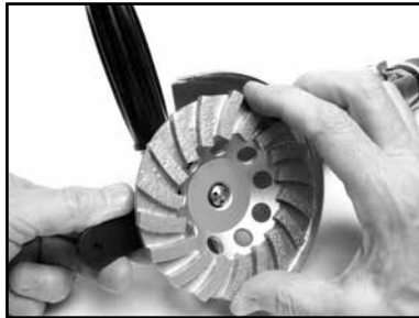
(K) Screw on Cup Wheel and tighten.
