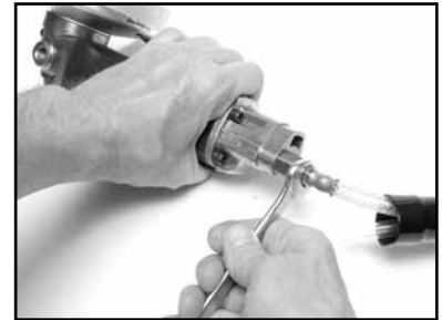
(C) Tighten the air hose nut.
