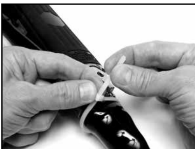
(G) Use the fastener to secure exhaust hose to grinder.
