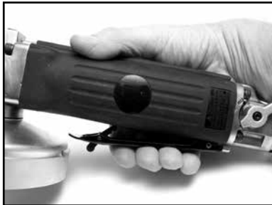
(M) Use handle to control air flow. Begin grinding.
