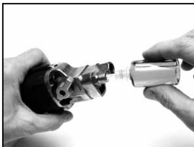
(A) Use 3-4 drops of spindle/machine oil in the air intake valve. The grinder must be oiled daily.
