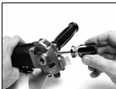
(B) Grease gears as needed using a multi-purpose EP lithium grease or moly EP lithium grease. DO NOT use oil.
