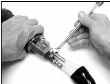
(E) Tighten the water hose nut.
