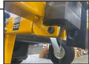
4. Secure the No Lift with Pins and Clips.
