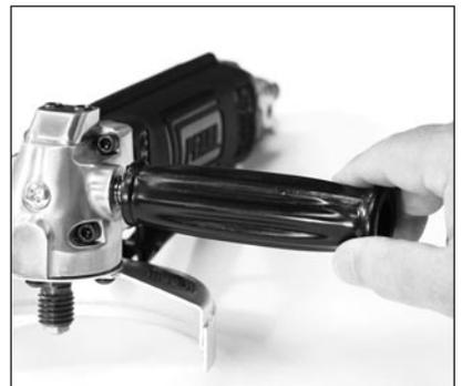
9. Attach the handle and tighten.
