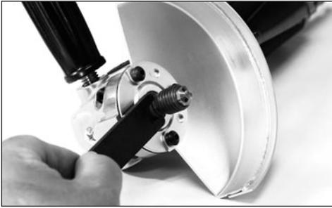
1. Place wrench on bottom of spindle.
