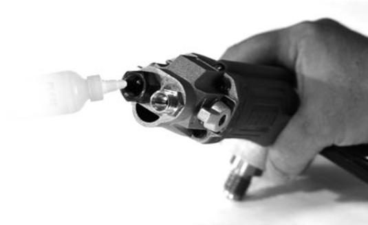
Grease gears as needed using a multi-purpose EP lithium grease or moly EP lithium grease. DO NOT use oil.
