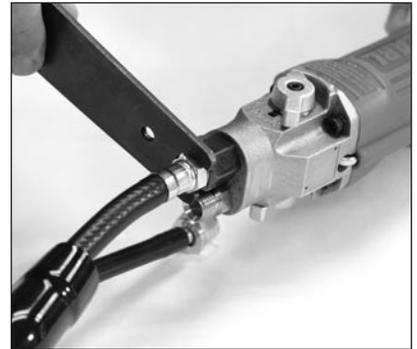
3. Tighten the air hose nut.
