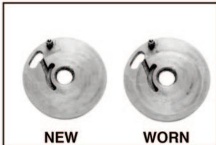
Wear in rear plate due to worn bearings.
