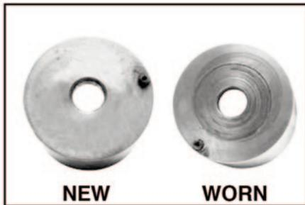
Wear in front plate due to worn bearings
