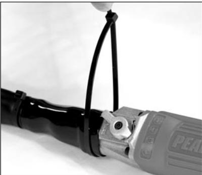
7. Use the fastener to secure exhaust hose to the grinder.
