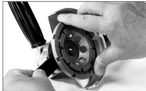
2. Screw on cup wheel and tighten.
