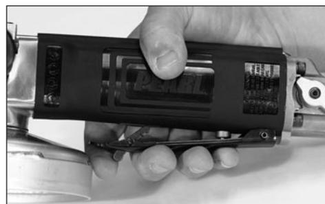
4. Use the lever to control air flow. Begin grinding.
