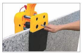
7) Before lowering the slab, make sure that there are no obstructions to disturb the slab to touch down on the stand.
