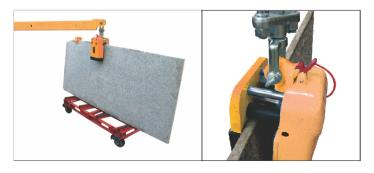
3) Unlock the locking latch so that the jaws will lock the slab when the lifting pin is raised through Swivel Shackle.
