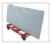
2) WARNING: Position the clamp squarely and in the centre of the slab so that the load is balanced. Make sure that the slab is inserted full depth into the opening of the clamps.
