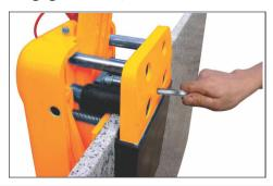
6) Before moving the slab to the desired position, move the slab close to the stand, lower the slab and keep a distance of about 10cm from the base, then unlock the safety lock (twist the safety lock anticlockwise).
