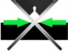
Adjust the two spindles so that the point at which the blades cross is at the top of the stone.
