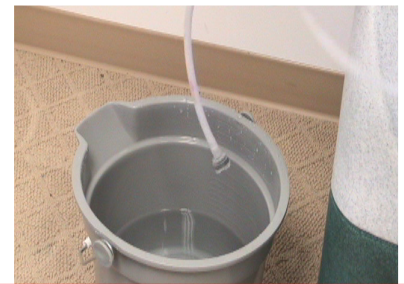
Place Chemical Feed Hose into Rinse Solution
