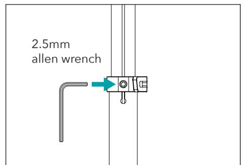
**OPTIONAL:** To ensure the handle will not move, tighten the set screw into the handle.
