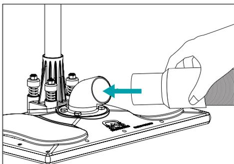
**1.** Connect vacuum hose from a portable or truck-mounted extractor. 2" cuffs will slide over the vacuum port and 1.5" cuffs will slide inside.
