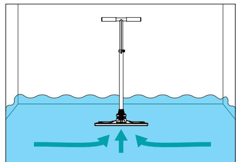
**3.** If there is standing water, place the SOS PRO in the center of the room to remove the standing water down to the carpet level.
