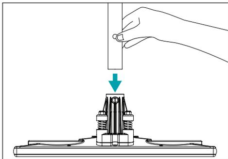
**1.** Press in the spring button and slide the handle into the handle base. Make sure the spring button lines up with the hole. It will snap into place.
