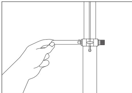
**2.** With the handle in place, pull the cam lock lever outward to loosen the clamp. Slide the handle up to desired height and press the lever back inward to tighten.
