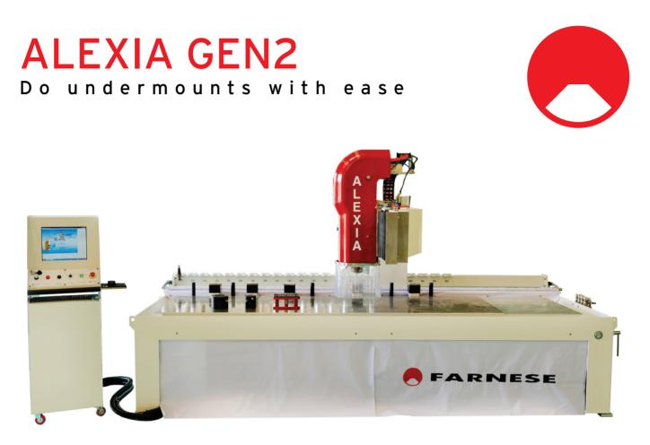
The ALEXIA automates the cutting, drilling and polishing of sink cutouts and is the ultimate answer to affordable stone processing without compromising on quality. The machine has automatic tool changing with 23 stations.
