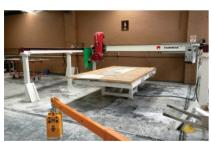
The LYNX is a saw designed and built for the person who needs an accurate and versatile saw at an affordable price. This machine is composed of one main beam (bridge), which travels on two rails. The main beam consists of one fabricated H beam on which 8 guides are machined to carry and drive the cutting head.
