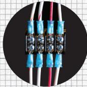
Plug-and-play wiring harness simplifies motor and pump replacement
