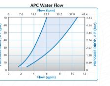
K These graphs are intended to give you a general idea of the performance capabilities of each product line. The shaded area of each graph represents the operating range of the product family, i.e., upper and lower values are shown. Therefore, depending on the exact coupling configurations selected, you can reasonably expect values to fall within the shaded area.
